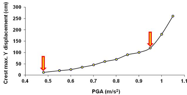
**Fig.10. Variation of crest permanent settlement versus PGA increase**
