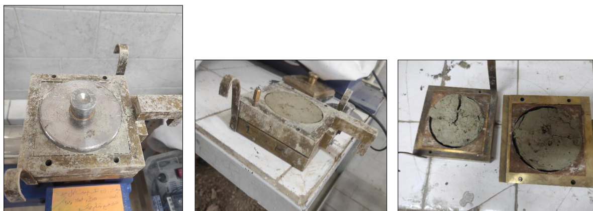
Fig.2. Images of the mold made and direct shear test of the samples
