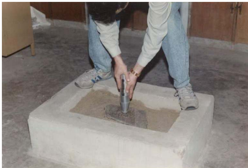
Fig. 1: Measurement of uniaxial compressive strength (JCS) by L-type Schmidt rebound hammer under saturated condition.
