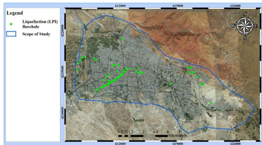
Figure2. Location of boreholes that have liquefaction potential in study area.
