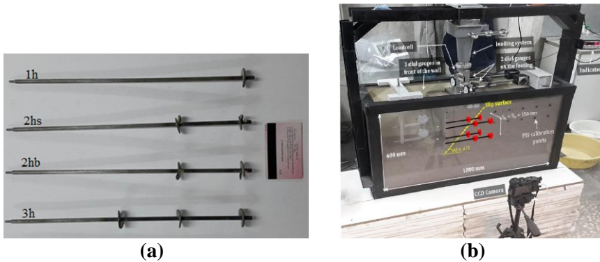
Fig. 4. (a) 4 Type of anchors used (b) Test box
