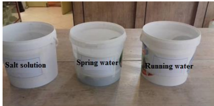
Figure 6. Solutions prepared for salt weathering tests
