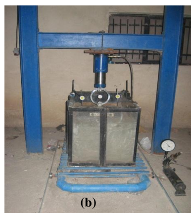
Figure 5. Vibratory tamper and test box during loading
