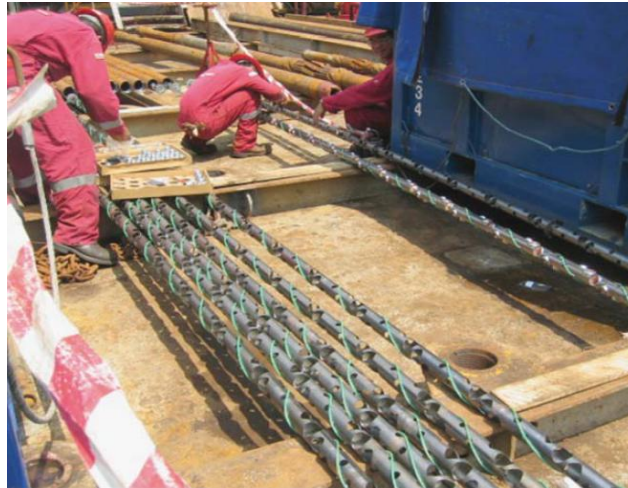
Figure 1. Loading shaped charges into perforating guns [6]
