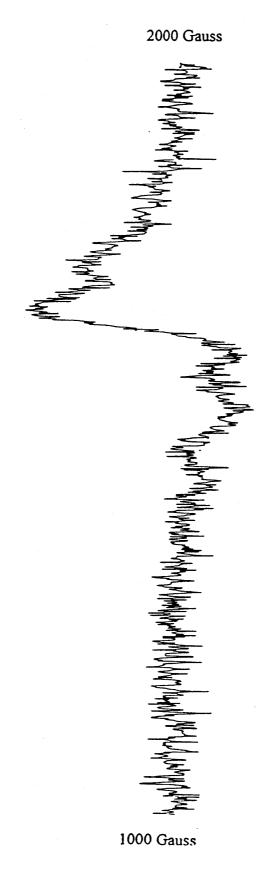
Figure 1: ESR spectra of complex [Cu<sub>2</sub>L<sub>1</sub>] at 135 K. The field set was 1500 gauss, and the scan range was 1000 gauss.
