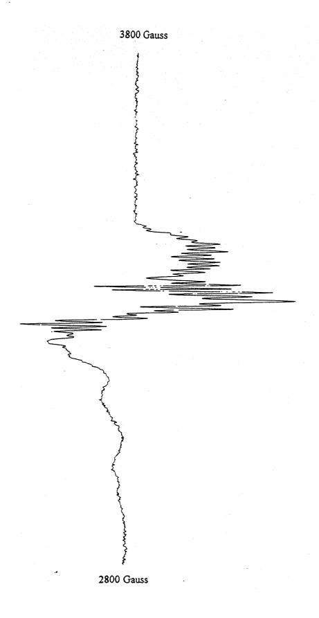
Figure 4: ESR spectra of complex [Cu<sub>2</sub>L<sub>2</sub>] at 130 K. The field set was 3300 gauss, and the scan range was 1000 gauss.
