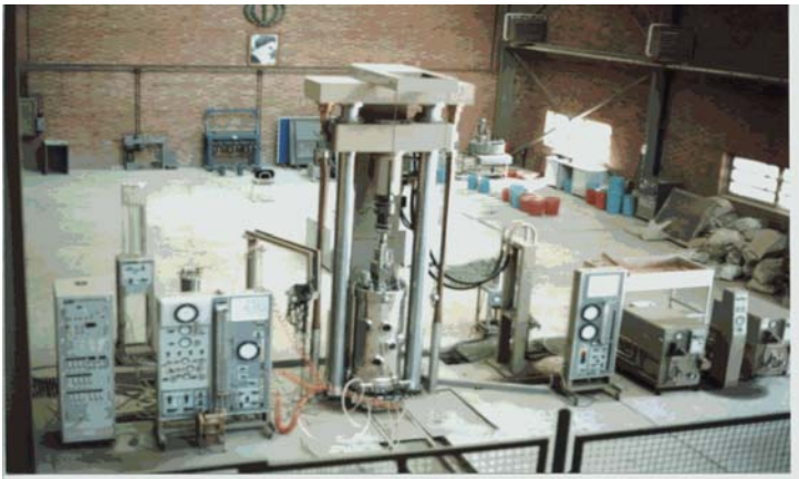
Fig 2. Large triaxial apparatus
