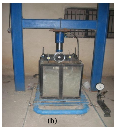
Figure 5. Vibratory tamper and test box during loading
