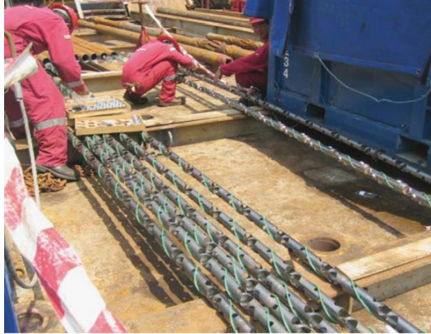
Figure 1. Loading shaped charges into perforating guns [6]
